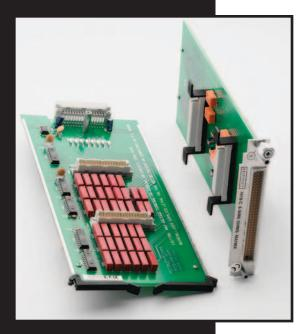
The Model 7019-C 6-Wire Ohms Matrix Card is specifically designed for automated production testing of resistor network devices in conjunction with the six-wire ohms function of Keithley's Series 2400 SourceMeter instruments and Model 7001 or 7002 Switch Mainframes. When these instruments are combined with the 7019-C in a production test system, the "per element" test time is typically less than 10ms, with maximum speeds typically less than 4ms.
